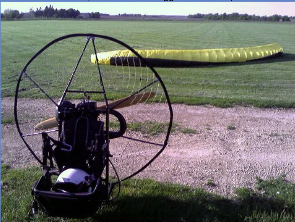
PHOTO 2: My motor with freshly welded muffler -- the welds at the muffler root appear to have done the trick (thanks for the suggestion Lance)
